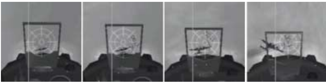
Fig 18. In the sequence above, a 110 is vainly trying to outzoom a Curtiss Hawk who cuts across his circle and fires a long burst from range 400 (first frame) down to range 200 (last frame). The amount of deflection and the effects are clearly visible.
