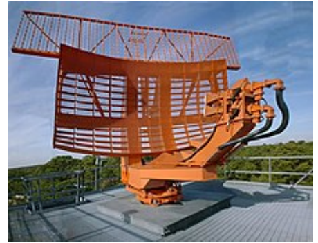
Secondary surveillance radar antenna ( flat rectangle, top ) mounted on an ASR-9 primary airport surveillance radar antenna ( curved rectangle, bottom ).
