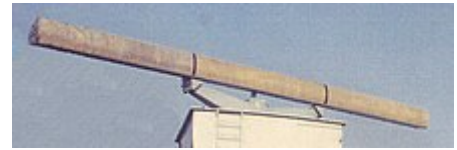
Original SSR antenna providing a narrow horizontal beam and a wide vertical beam
